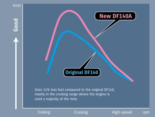
Data used in the graphs were obtained through in-house testing under unformed conditions. Results will vary depending upon operating conditions (boat design, size, weight, weather, etc.)
